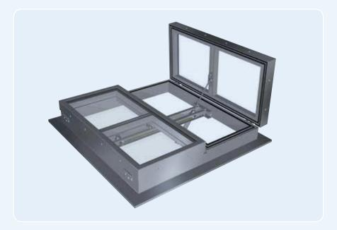
The cold bridge-free Duo Therma TG fitted with a thermally separated base and flaps offers a high level of durability. It minimises condensation forming and offers advanced comfort features. In the event that sound insulation is also required, two fully acoustic versions of the Duo Therma TG model are available, which have Rw values of 34 dB and 44 dB, and are fully compliant with the EN 12101-2 standard.
